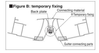
4 Fix the gutter connecting parts to the back plate inserted into the connecting material with small truss screw  $5\times15\times10$ .
