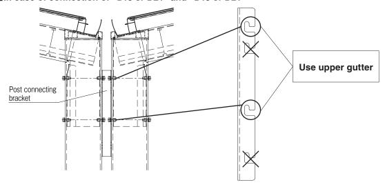
■In case of connection of "Any side from D24 to D33" and "Any size from D24 to D33"
